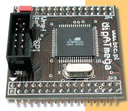
ZL7AVR is an easy to use versatile mini-module based on Atmels ATmega128 microcontroller (AVR enhanced RISC architecture). In ZL7AVR module all ports and signals of the microcontroller are available on two-row pin connectors with 0.1' pitch (pin headers). In addition, we offer prototype board ZL8AVR.
