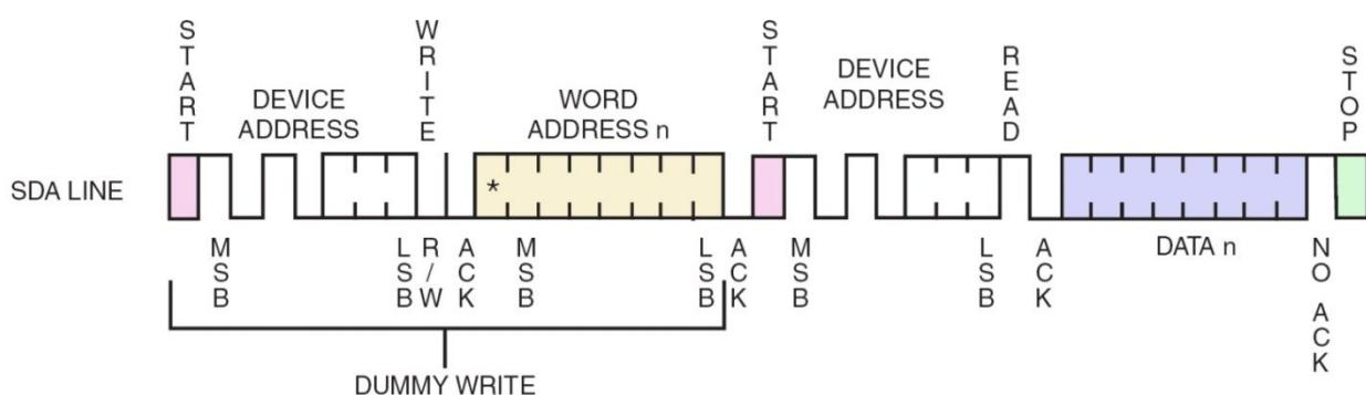
**Medium and High Density Random Read:**
