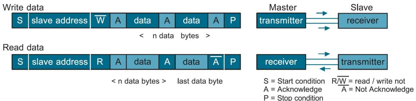
A write operation requires a device address bytes, two address bytes and the data-byte. Upon receive of the address the EEPROM sends an ACK and then clocks in the data-byte. The EEPROM sends again an ACK and the microcontrollers sends a stop-signal to terminate the write sequence.
