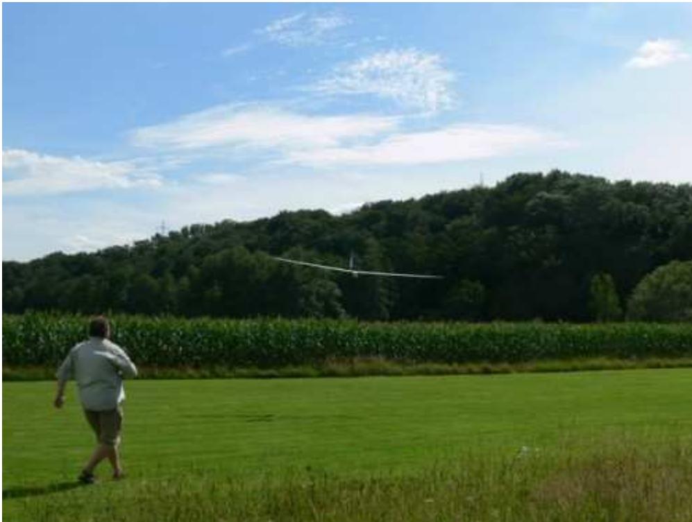
Fig. 2: Hand launching a 4m Alpina (6.5 kg) is always a thrilling exercise. Luckily it worked out – not only one time: The 2009 season saw a total of 29 successful Alpina flights using the AR7212-DX7 combo. Not a single failure or malfunction during about 15 h of flight.
