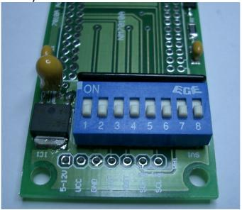
Finish with soldering the NM7010A module. The header pins are optional.
