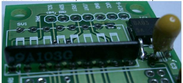
Finally solder the DIP switch.
