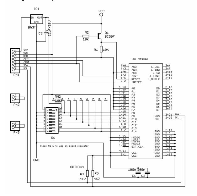
The 4K7 pull up resistors are optional and not mounted.
