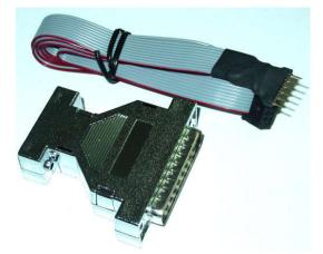
Another interesting option is to use an AVR-ISP Parallel Port programmer and software available in **Bascom-AVR** by **MCS Electronics**, as shown in adjacent images. This programmer is adapted for development. The schematic diagram of this programmer can be found in the Bascom-AVR Help files.
