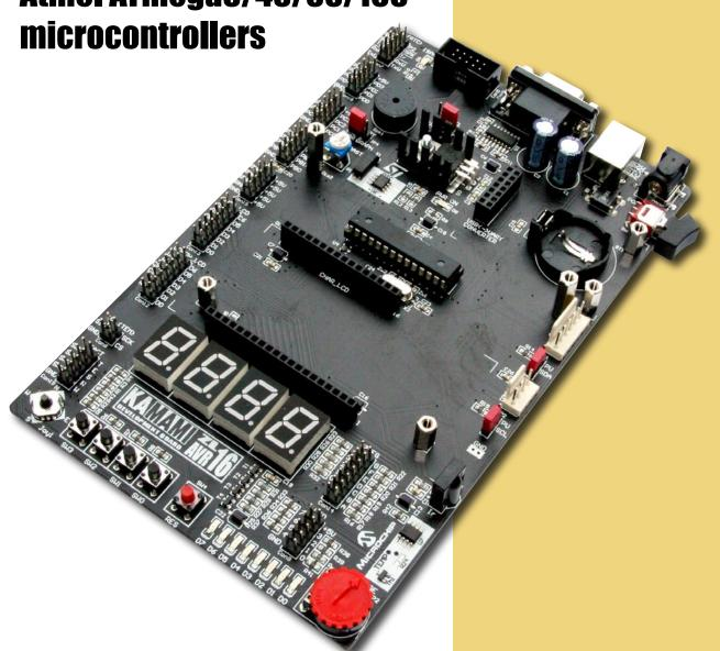
ZL16AVR is an universal development board for ATmega88 (and other AVR microcontrollers in 28-pin package, like ATmega8/48/168). With a wide range of peripherals it can be used as an environment for development of prototypes or as an education board.
